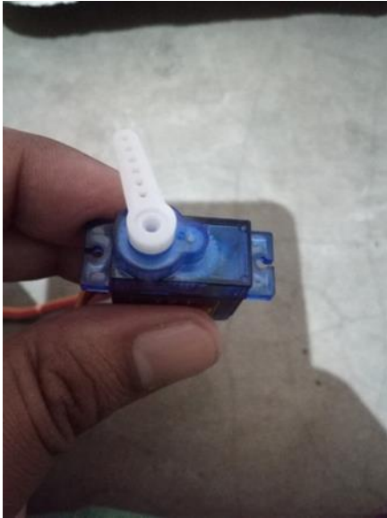
Fig. 10 Servo motor angle movement to 90^{\circ}
